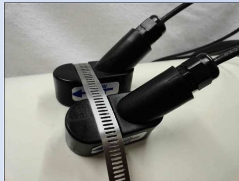
Figure 3. Clamp-on transducers secured with a SS 1/2" gear clamp band
